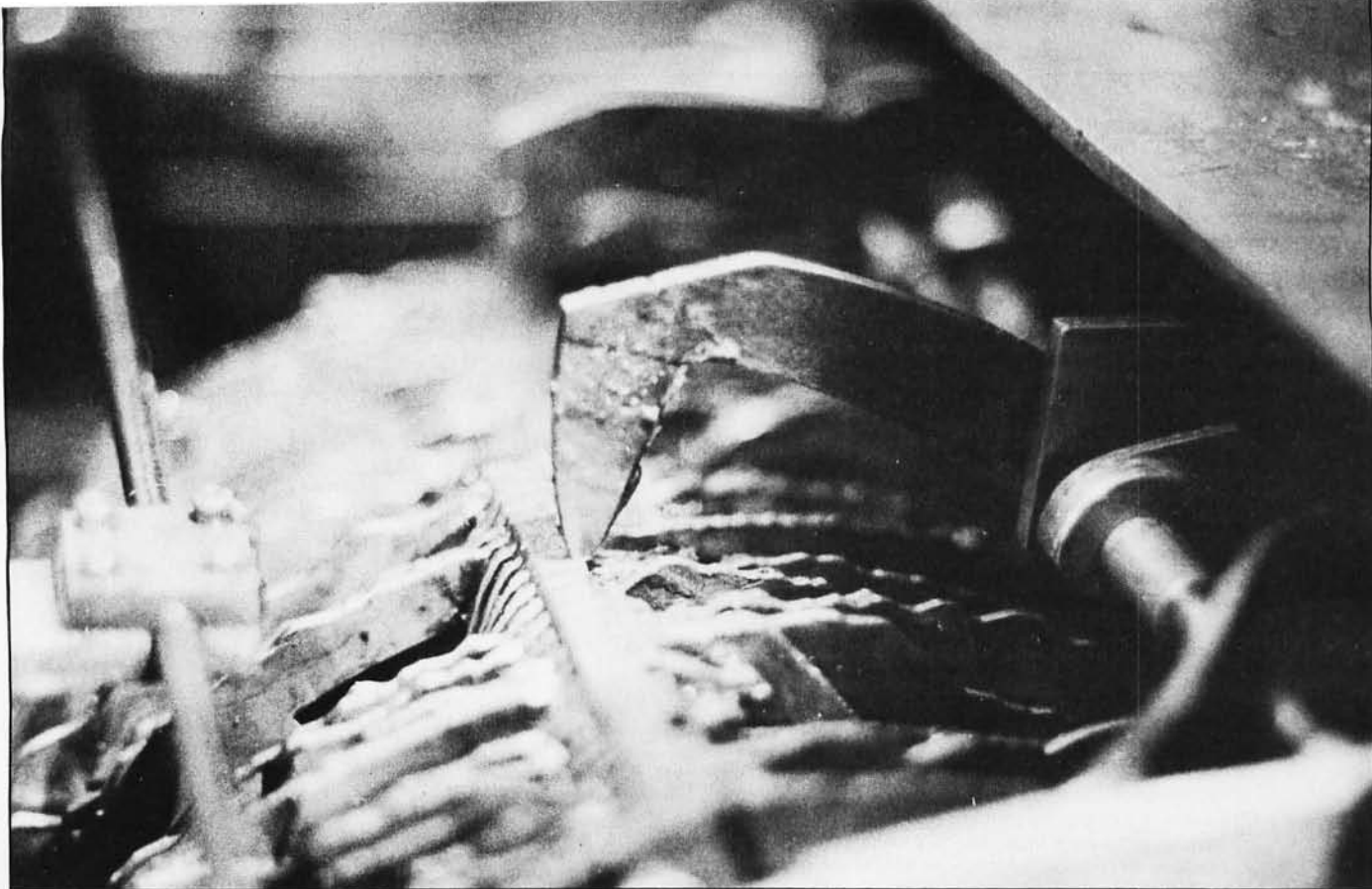
Photo 5: Center follower at rest on the bar on which it slides as the cam deck is positioned laterally. The undulations of the cams are also visible.
