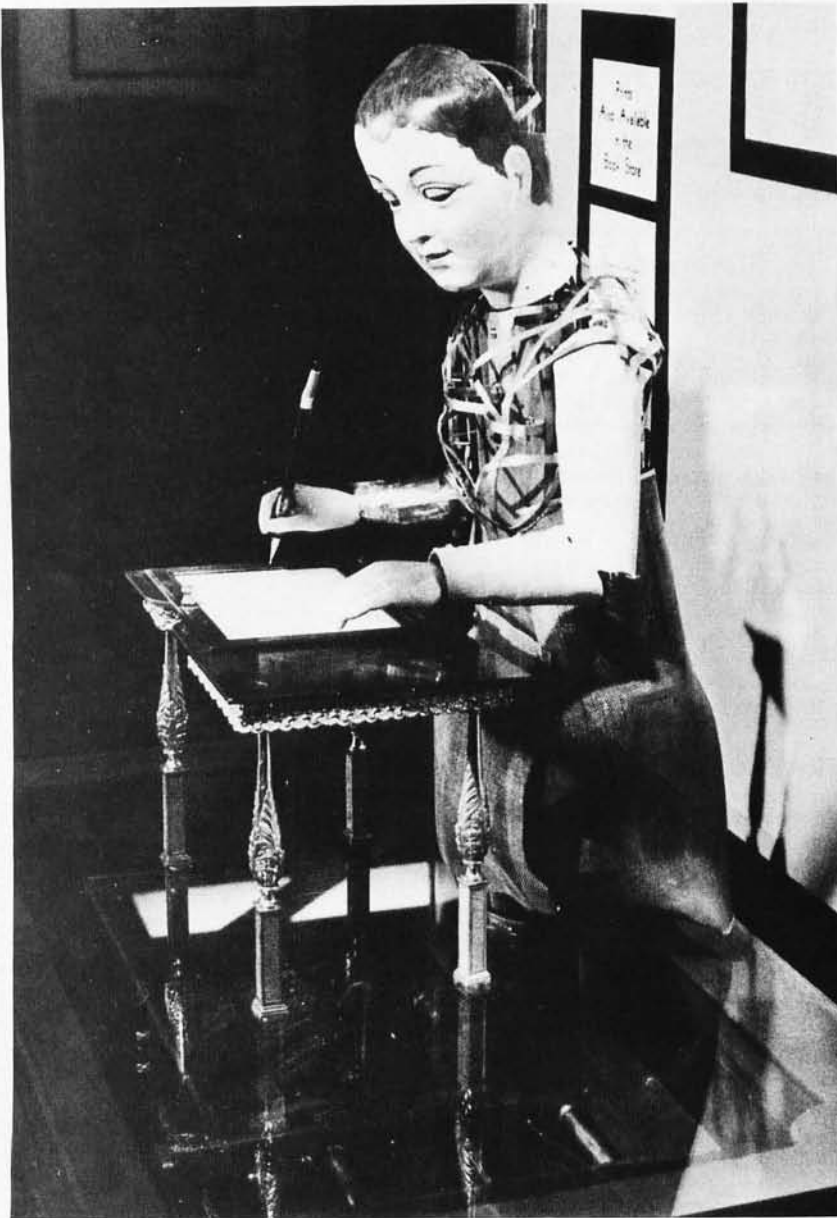
Photo 3: The Maillardet writing and drawing automaton sans clothes. The body of the figure is made from strips of brass and wire; the glass floor reveals the mechanism. A modern pen is shown in the automaton's hand. Courtesy Franklin Institute.
