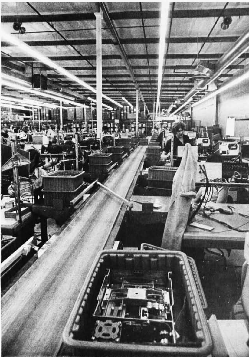
Photo 1: One of the high speed conveyors at Shugart Associates' Sunnyvale CA plant. Metal arms swing out to capture plastic bins of parts. 600 to 800 floppy disk drives and 300 to 400 minifloppy drives are turned out every day at the plant.
