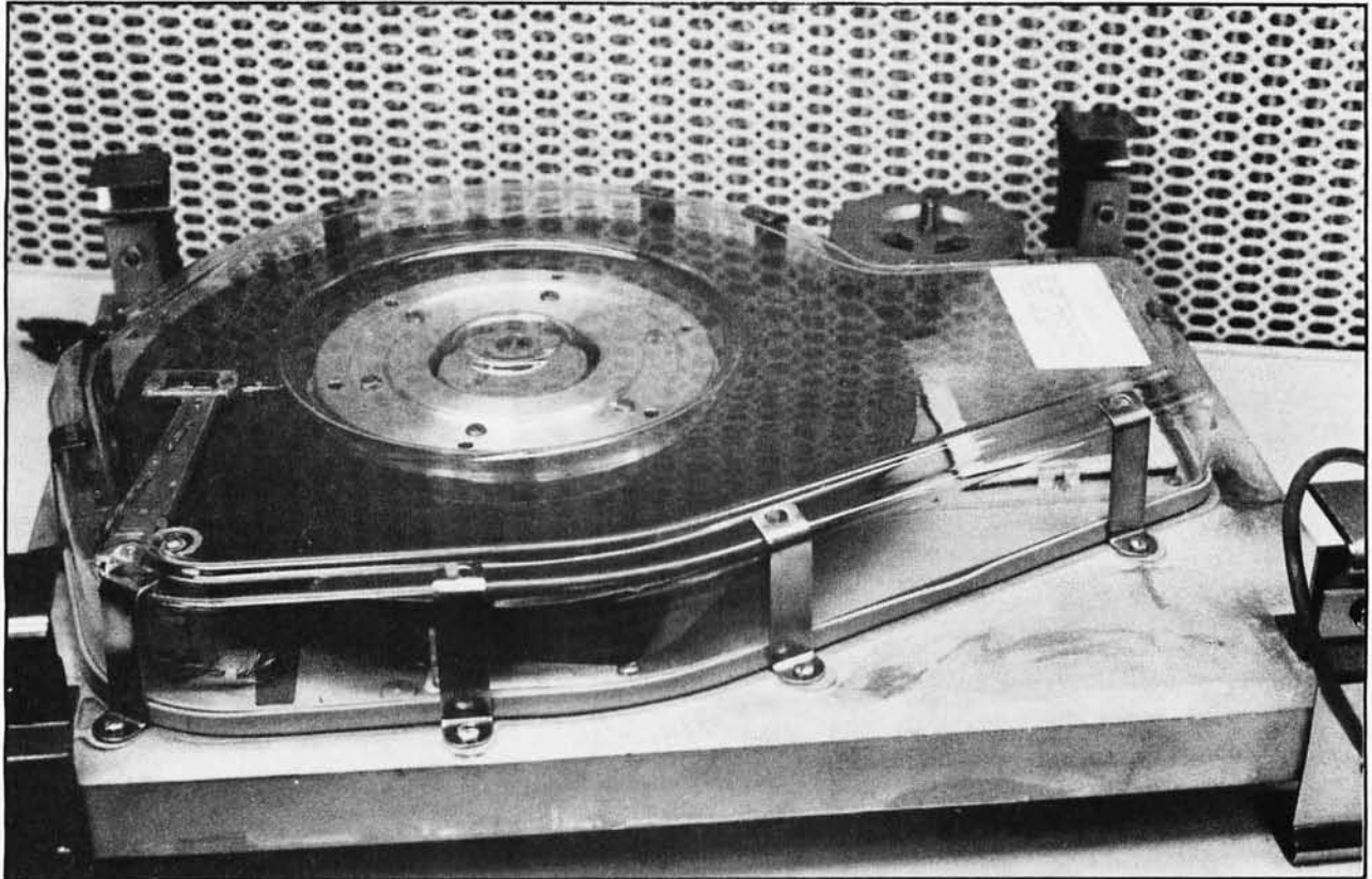
Photo 2: Prototype of the SA4000 fixed disk.
