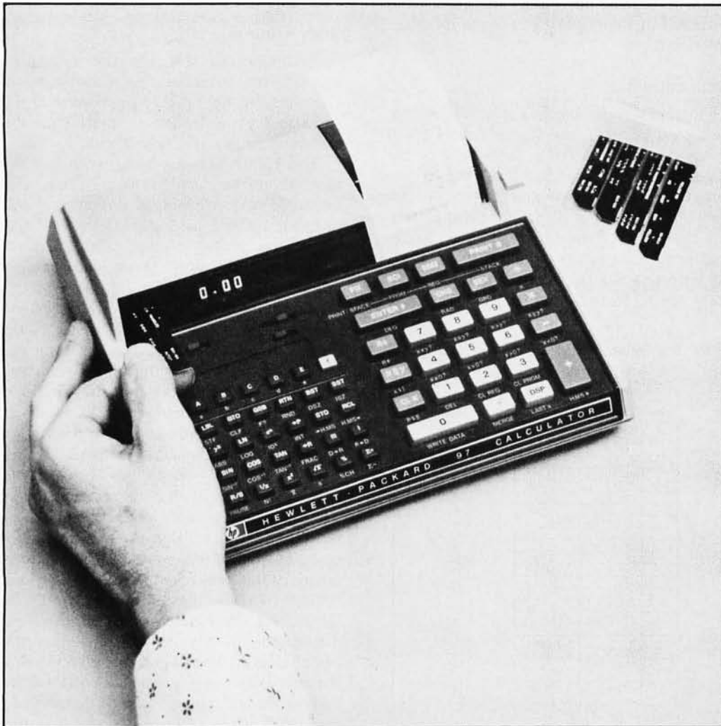
Photo 2: The Hewlett-Packard HP-97 programmable desk top calculator with printer. (Photo courtesy Hewlett-Packard Co.)
