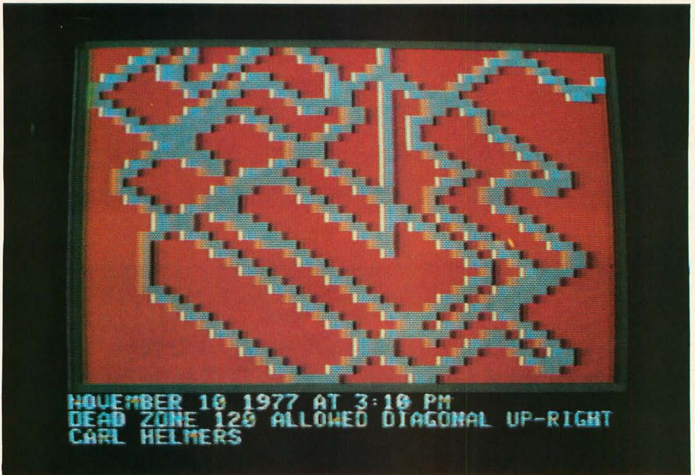
Photo 6: An example of another product of the color sketchpad program, in this case illustrating a text tag entered by the program's "T" command to identify when and who did the illustration. The comments on the second line of the text at the bottom refer to an experiment with the program's joystick dead zone parameter.
