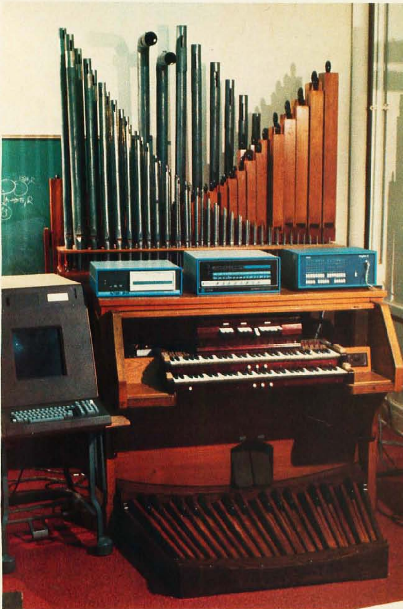
Photo 1: The authors' overall system with graphics terminal on the left and the disk drive and two computers on top of the organ console. The wooden pipes at top right are the flute rank; the metal pipes are a viola rank. The stop tablets for selecting ranks and harmonics can be seen just above the top keyboard.
