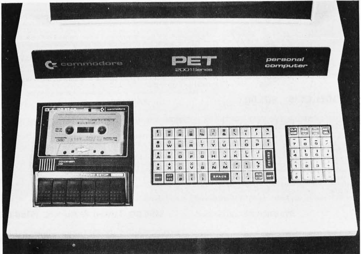
Photo 2: A close-up of the PET keyboard and cassette drive. The keyboard is a flat, calculator style unit with 73 keys. The upper case shift positions on 64 of the keys are occupied by graphic characters. At the right are the cursor control and insert/delete keys and a numeric keypad.
