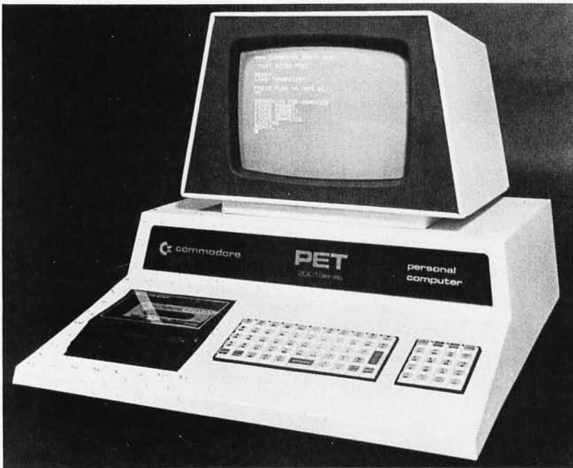
Photo 1: A view of the Commodore PET, Model 2001. This personal computer sells for $595 and includes a keyboard, video display, cassette drive, 4 K bytes of programmable memory, and a BASIC interpreter and operating system in 14 K bytes of read only memory.
