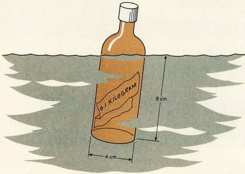
Figure 1: A bottle sinks until it displaces an amount of water equal to its own weight.
