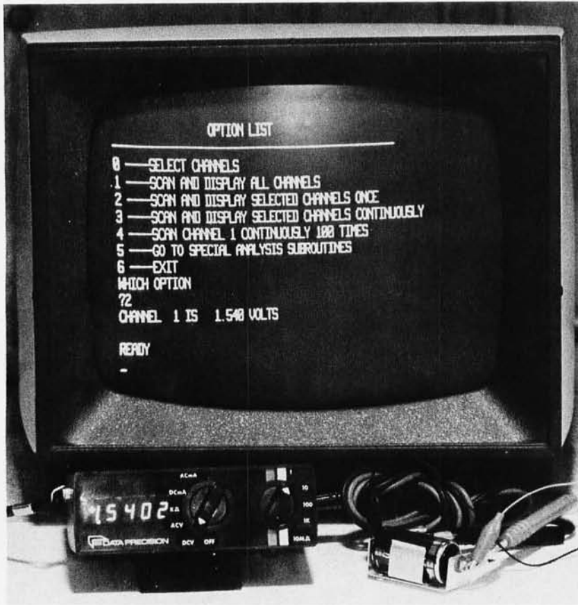
Photo 4: An illustration of the accuracy of the computerized voltmeter. A Data Precision 4½ digit digital multimeter and the author's system simultaneously measure a C cell battery. The computer value is 1.540 V compared with the Data Precision reading of 1.5402 V.
