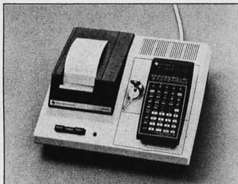
Photo 2: The TI 58, shown mounted on the PC-100A printing cradle with alphabetic printing capability.
