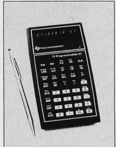
Photo 5: The new TI 57 programmable calculator can store up to 150 keystrokes.
