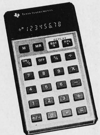
Photo 8: The TI 1680 replay calculator, which remembers the last 20 numbers and operations entered, is useful for checkbook balancing.
