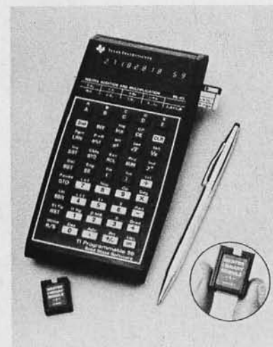
Photo 4: The TI 59 features Solid State Software plug-in program library modules of up to 5000 program steps, as well as a magnetic card reader and internal memory for 960 program steps.
