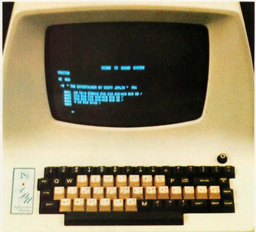
Photo 2: The modified ADM-III video terminal. The keytops on the ASCII keyboard have been modified to enable the user to easily encode musical compositions. See figure 1.
