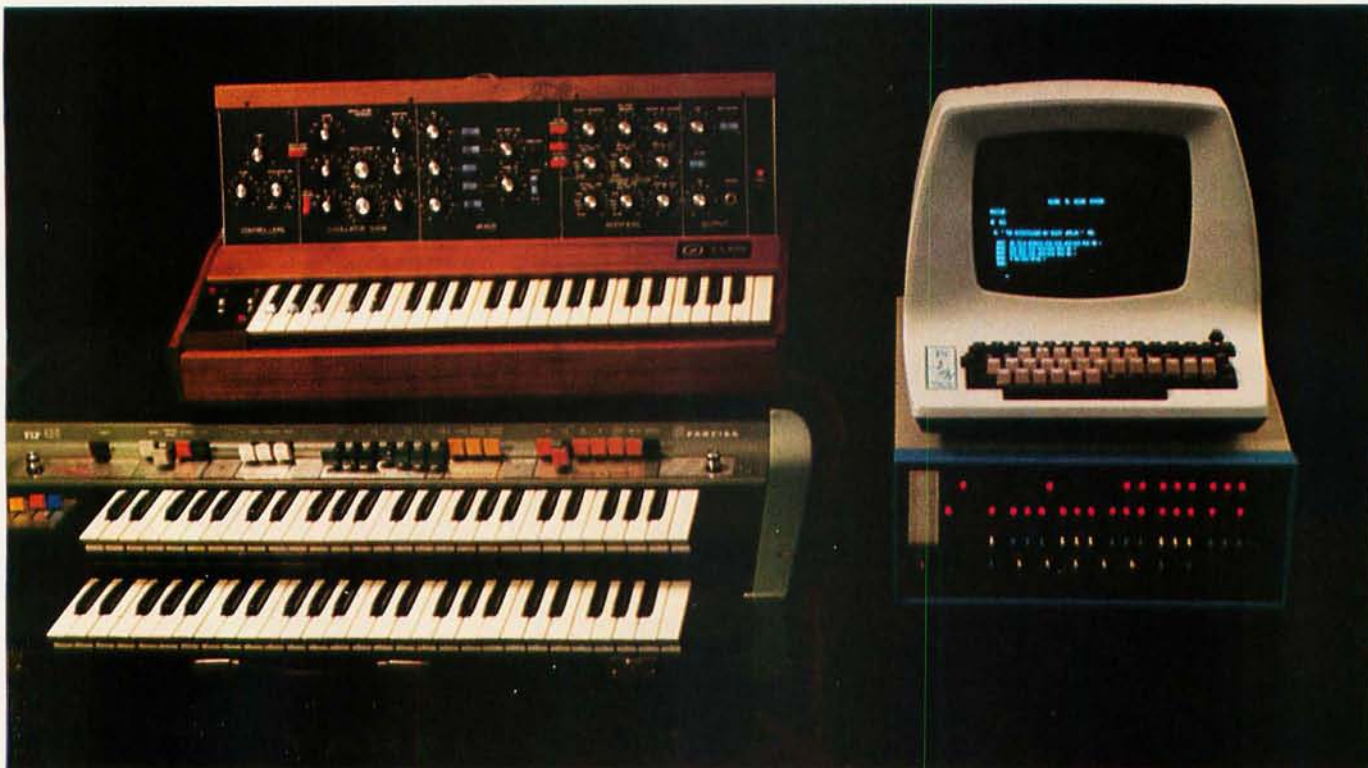
Photo 1: The author's computer music system, which consists of an Altair 8800 computer with 32 K bytes of programmable and read only memory, and an ADM-III video terminal. Also pictured is a Mini-Moog electronic music synthesizer (top left) and a Farfisa VIP 400 electronic organ (bottom left).
