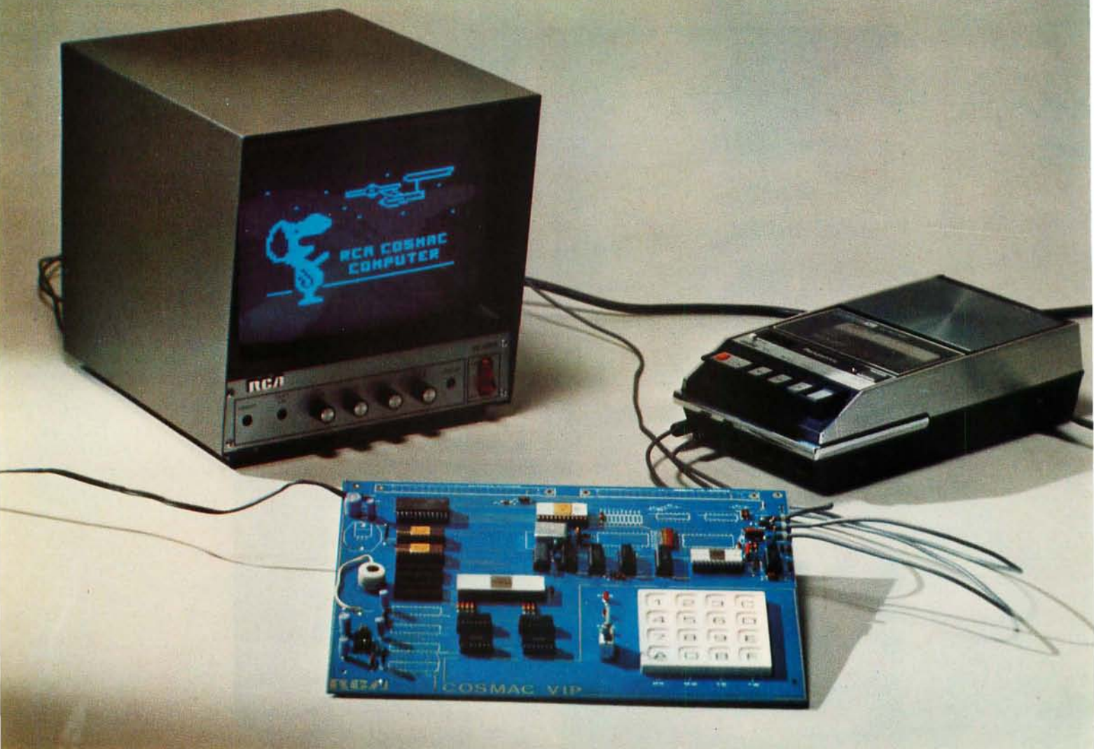
Photo 1: The COSMAC VIP system demonstrating its graphics abilities. The kit version of this product includes the board alone; the user must supply a standard video monitor (or modified TV) and inexpensive tape recorder.
