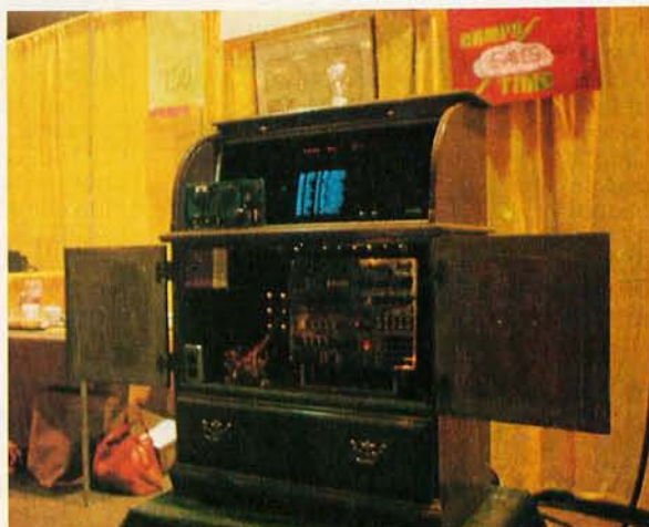
Photo 2: The mild, unassuming roll top desk at the left of this sequence hides an intelligence. For, when all the doors and slides of this "desk" by RDC Enterprises (8352 Stanford Av, Garden Grove CA) are opened, they reveal an experimenter-oriented computer with built-in Altair bus extender card at desk level, a keyboard at desk level and video monitor. The actual computer mainframe is below desk level behind doors, and the bottom drawer can hold the experimenter's tools.
