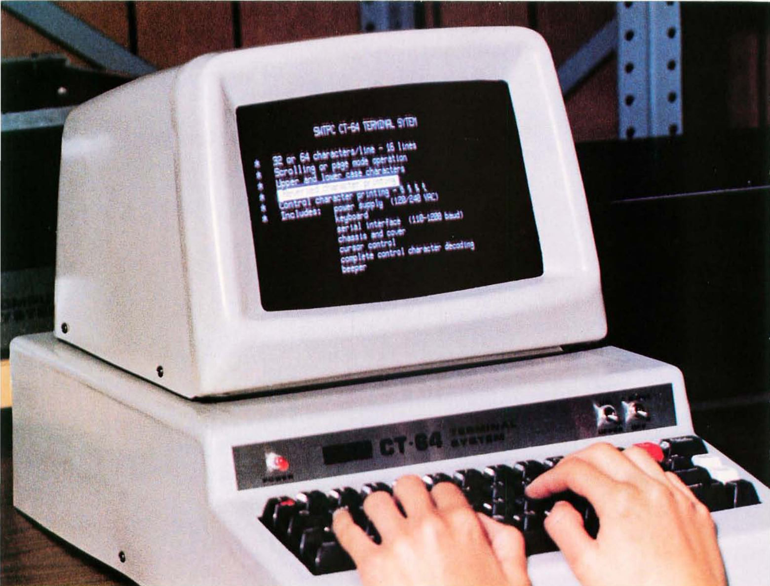
The 9-inch screen of the CT-VM monitor ($175) shown here with Southwest's new CT-64 illustrates the terminal's 64-character lines, switchable control character printing, and word highlighting. At just $500 for both, these matching units provide a complete CRT terminal with full cursor control, 110-1200 Baud serial interface, and many other features.
