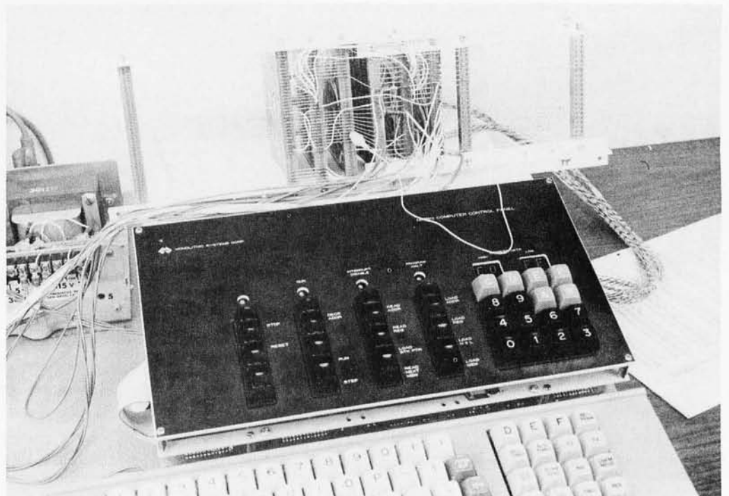
Photo 7: Physical layout of the equipment. The author's display is shown here as it was built on prototyping cards with a bus wired backplane between connectors. The clip lead is shown here attached to memory address bit 7, as used to generate photo 3. The computer and keyboard are in the foreground.
