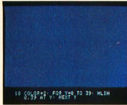
Photo 2a: The first step in any game is to generate the uniform color background for the action of the game. Here we use a blue field.
