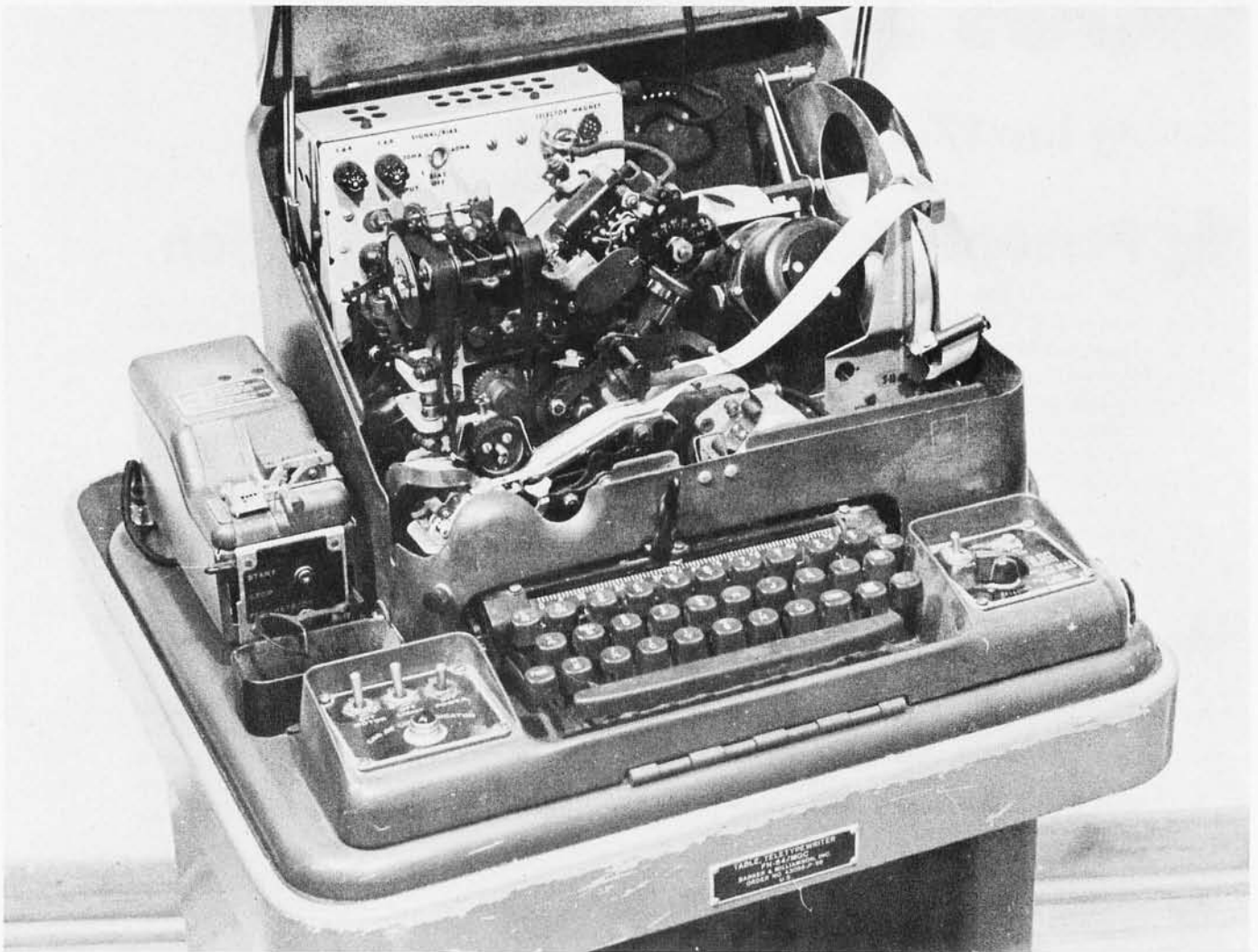
Photo 5: A view with cover lifted of the author's Kleinschmidt Model TT-76A (military nomenclature). This machine is a paper tape punch and reader only, which actually types characters on the tape. Like the Kleinschmidt in photo 4, this unit contains a loop power supply.
