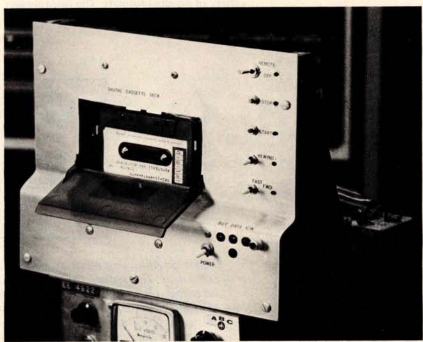
Photo 2: Ira Rampil's homebrew mount for the Phi-Deck mechanism he will be using with his PDP-11/20 system as a mass storage file subsystem.
