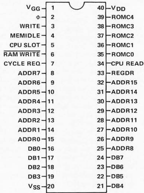
Figure 8: Pin designations for the 3853 static memory interface chip.
