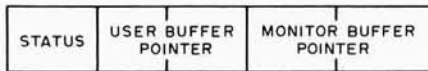
Figure 3: Buffer Control Block. When buffering is used to allow overlap of processing with IO operations coordinated by interrupts, a buffer control block consisting of two pointers and control flags can be a useful construct. In the ELM case, the first two byte pointer is set to the address of the current user buffer, and the second two byte pointer is set to the address of the current monitor buffer used by the IO routine. The flag called STATUS in the first byte of this five byte control block example is used to coordinate the IO tasks with the user's program.
