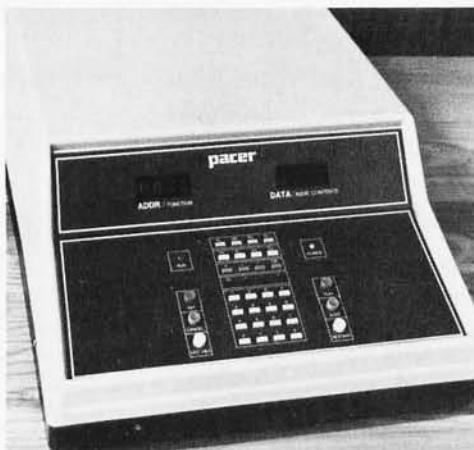
Photo 1: When assembled, Pacer is a neat desk top package with a molded plastic case and calculator style keyboard. The dot matrix alphanumeric display is here shown as it appears when the Pacer is initialized by pressing the INT button.
