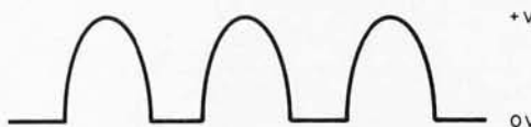
Figure 8: Voiced Sounds from the Glottis. Sounds which have definite pitch are called voiced sounds. In the natural larynx, these sounds are generated by the vocal chords and drive the vocal tract at the glottis. In an electronic analog, the voiced sounds can be generated by a programmable counter (to set the frequency) which in turn creates a sine wave of the same frequency. A rectified sine wave is a good source for the glottal pulses used in the electronic model of a larynx used in the author's approach to speech generation.
