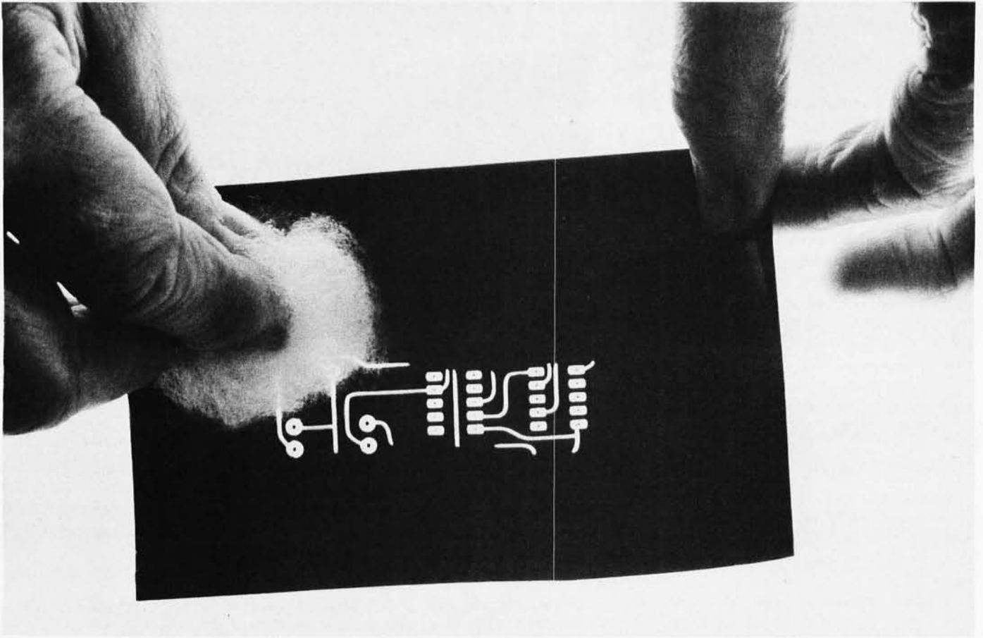
Photo 7: Creating a Photo Negative for Etching. A negative is reproduced from the positive artwork pattern, using a reversing film. The film is exposed with a bright light, then developed by rubbing gently with a cotton swab and developing solution. The result is a negative version of the artwork with a 1:1 scaling.
