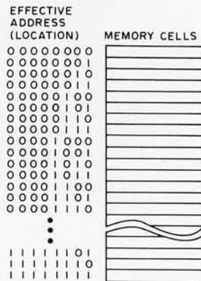
Figure 1: Memory Addresses. The effective address is the object of memory address calculations. It identifies a location in memory address space for the particular cell involved in some operation.
