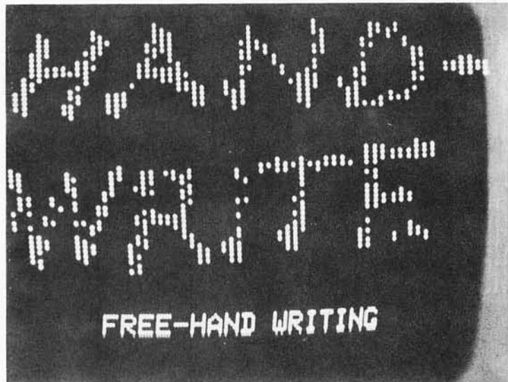
Photo 3: The light pen can be used in an "enhance" mode by using a footswitch control to flood the screen momentarily when the light pen is in position.
