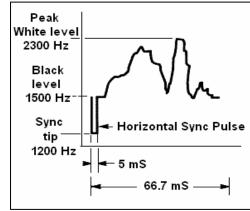
invisible. The sync pulses that are sent at the end of each line are 5ms in length and at the end of each frame 30ms in length.
