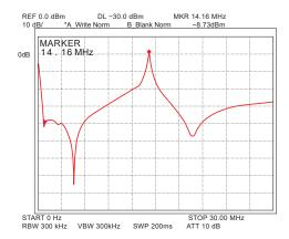
Figure 01-02: Filter Characteristics of Digi-Sel
