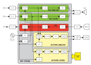
Figure 02-04 FPGA Internal Block Diagram and ROM
