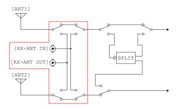
Figure 01-08: RX-ANT IN/OUT switching circuit block diagram
