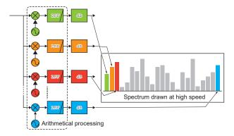
Figure 02-07 FFT operation diagram (equivalent)
