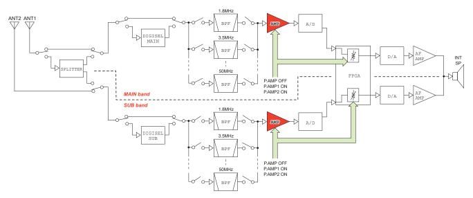
Figure 03-02 Receiver block diagram showing preamplifiers & downstream gain-distribution adjustment
