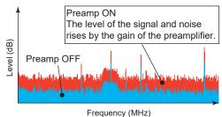
Figure 03-03: Preamplifier operation (conventional method)
