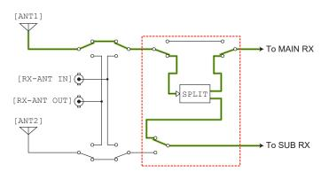
Figure 01-11: Signal path when ANT 1 is used in both bands
