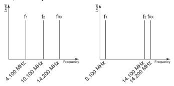
Figure 01-04 Second-order intermodulation distortion examples
