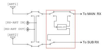
Figure 01-10: Splitter circuit block diagram
