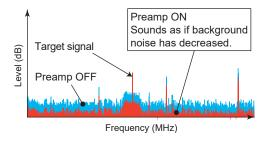
Figure 03-04: Preamplifier operation in IC-7610.
