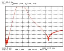
Figure 01-05: BPF Characteristic for 11.0 ~ 14.999 MHz Band
