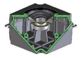
Figure 03-01 Speaker box of IC-7610 (sectional view)
