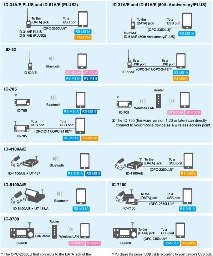
transceiver is supplied the two types of USB cable, for an Android device (USB mini-B/USB micro-B) and a PC (USB mini-B/USB Type-A).
